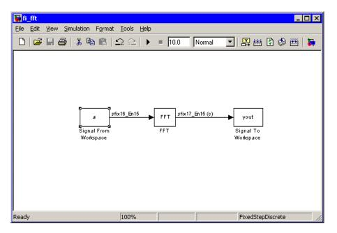
The Signal To Workspace block writes the result of the simulation to the MATLAB workspace as a fi object.
