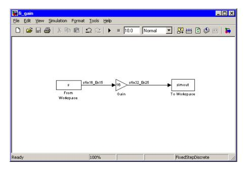
The To Workspace block writes the result of the simulation to the MATLAB workspace as a fi structure.
